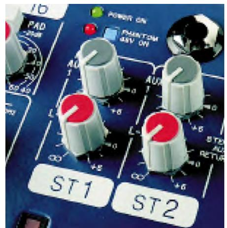
The WZ16:2 stereo inputs give you no-nonsense control over sources like 2-track recorders and stereo effects returns. You'll easily handle instant live-recording replays, interval music from CD, AV or other sources, helped by the mixer's comprehensive monitor and cue circuits.
