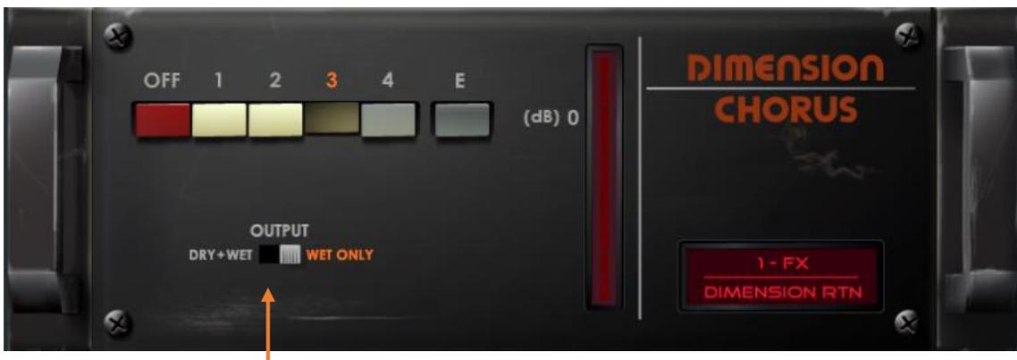
Set to WET ONLY when using in a Send/Return configuration, or 'Dry+Wet' when inserted.
