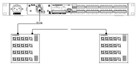
A DX Hub can be connected to the SLink card for further expansion with up to 8 DX expanders. It also enables a single cable link to the AHM processor in cases where multiple expanders are located on a different floor, area or building.
