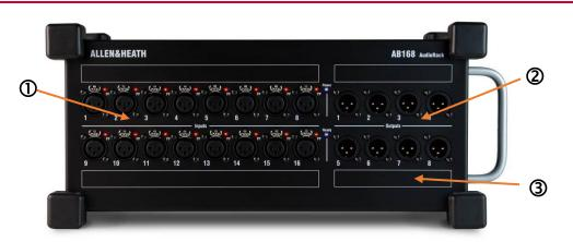
**(D)** Input sockets 16 balanced XLR mic/line inputs with +48V Phantom Power indicator. The preamps are built into the AB168 and their Gain, Pad and 48V phantom power are controlled remotely from the mixer via the dSNAKE link. The Phantom Power indicator detects voltage at the socket whether supplied by the AB168 or received from an external source. Refer to mixer documentation for information on patching these sockets to input channels or other destinations in the system.
