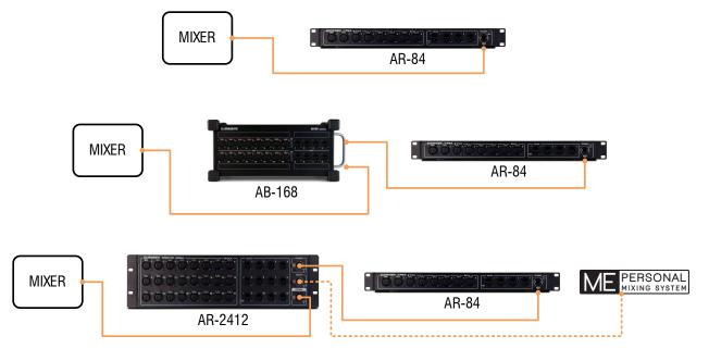
() A maximum of two dSnake remote units can be connected to each mixer's dSnake port.
