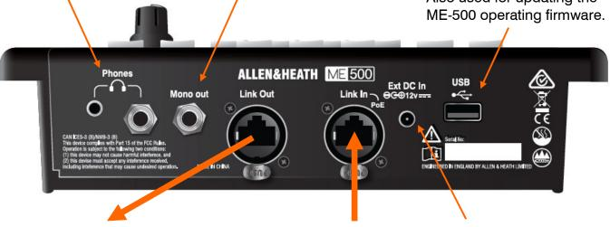
Link Out - Locking EtherCON connector to plug a Cat5 cable to feed audio to the next ME mixer when daisy chaining them together.
