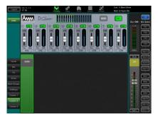
**Automatic Mic Mixing (AMM)** – This is very useful for speech applications such as conferences and seminars involving several microphones around a table. The Qu AMM can automatically take over the level of these mics to improve clarity and reduce the risk of feedback caused by many open microphones.
