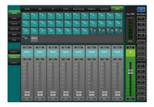
**USB B Streaming** – Connect an Apple® Mac or Windows® PC computer to the USB B port to stream up to 32 channels of audio in both directions and send MIDI messages.
