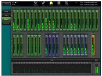
**RTA** – The built-in real-time analyser provides a useful display of the frequency response of the currently selected PAFL signal. This can help in finding problem frequencies in a room or while ringing out monitors.
