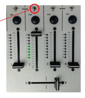
• Turn the corresponding channel fader up and monitor the LR MIX output (via headphones, MST, or BOOTH output)
