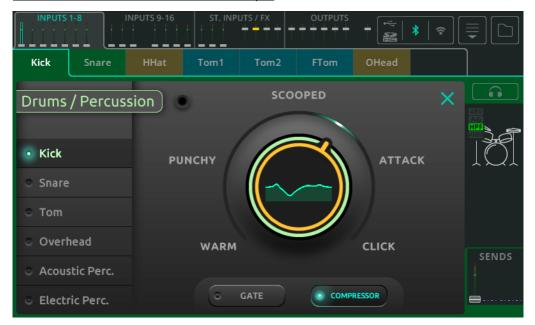
A 'one knob' Quick Channel has instrument or source types on the left-hand side.
