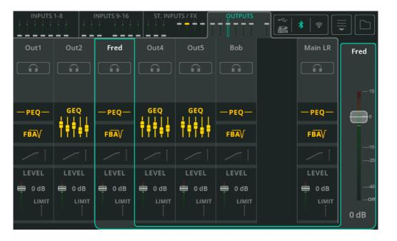
The Outputs bank includes the six Outputs and Main LR processing channels.
