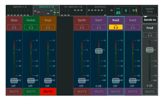
Touch **Sends to** and select an output to show all send levels to that output on the fader for each input and FX channel.
