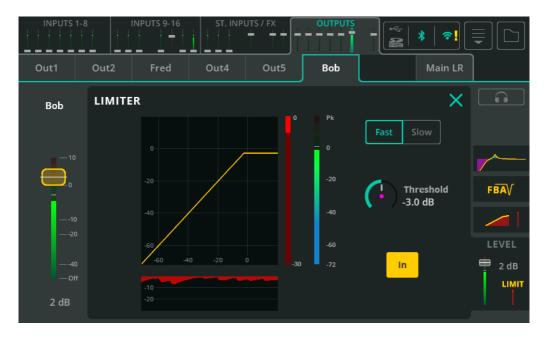
A Limiter works like a very fast compressor with an infinite:1 compression ratio and limits the output level to whatever is set by the threshold.
