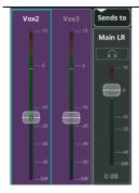
Raise the fader for any Input (or multiple inputs) to send signal from input channel to the Main LR output. Touch/Click and drag, or select the fader and use the Touchscreen rotary control (CQ-12T, CQ-18T).
