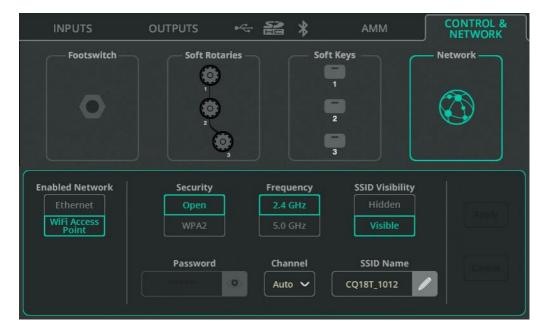
**Enabled Network** – Select **Ethernet** for wired connection through the Network port. Select **Wi-Fi Access Point** for wireless connection using the integrated access point of the unit (CQ-18T, CQ-20B).
