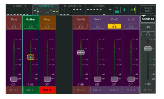
Touch **Sends to** and select an FX to show all send levels to that FX unit on the fader for each input and FX channel.
