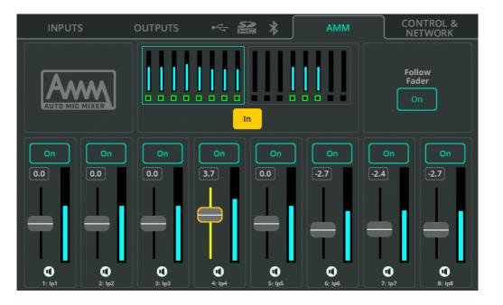
CQ's Automatic Microphone Mixer uses a gain sharing algorithm, designed for use in multi-microphone speech applications like conferences, meetings, broadcasting and podcasts. It can be used on every mono input channel of the CQ with two banks shown at the top of the page.
