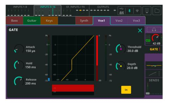
A Gate allows wanted signal through and attenuates unwanted signal. It has many uses including removal of hum from an idle instrument or avoiding hearing the snare drum through a tom microphone when only the snare is being played.
