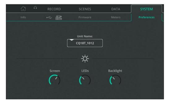
**Unit Name** – Change the name of the unit, as displayed in the 'Choose Unit' connection screen when using remote control apps (CQ-MixPad, CQ4You)
