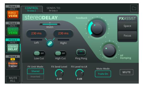
Stereo Delay includes two tap delays (left and right) where the speed of repeats can be set independently for each.
