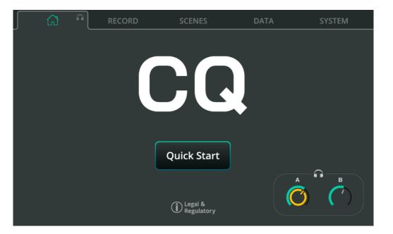
**Quick Start** – Recall mixer configuration and channel processing for different applications. See the Quick Start section for more information.
