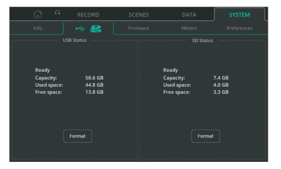
Displays details on any connected USB drive and/or SD Card
