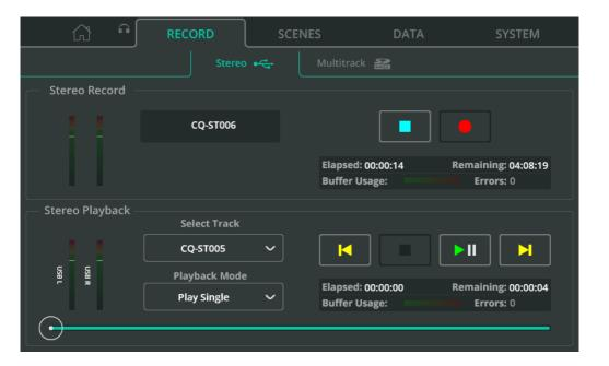
Stereo recording/playback to/from a connected USB drive.
