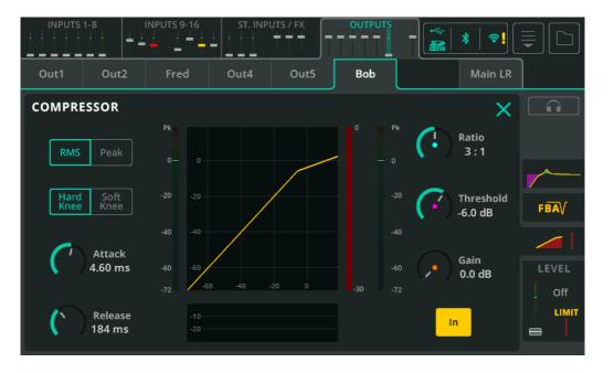
A Compressor is used to control and reduce the dynamic range of the signal.
