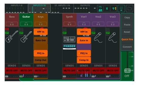
Open the dropdown menu from the top right-hand corner when in a bank view and select **Quick Fire** to view an overlay which allows processing to be quickly switched in or out across all visible complete channels.
