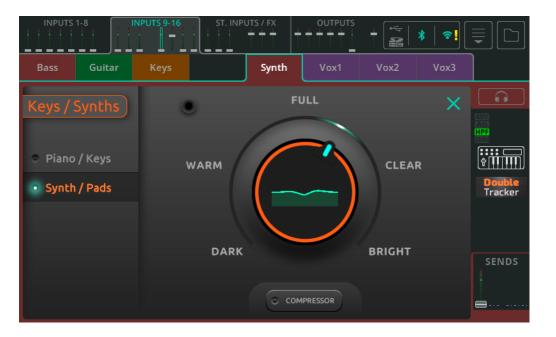
CQ includes Quick Channels for a variety of common audio sources which provide a quick and easy way to adjust multiple channel processing parameters with a few controls. This enables the mix to be put together much faster than with conventional controls and if more control is required, Quick Channels can be converted to Complete Channels at any time.
