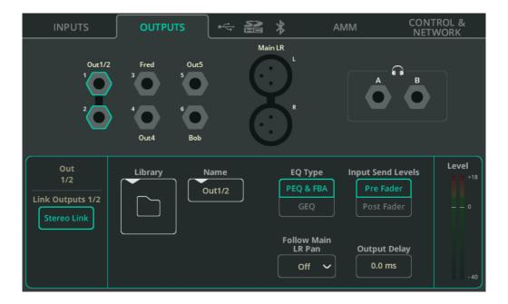
Output sockets are shown at the top of the screen, matching the hardware layout.
