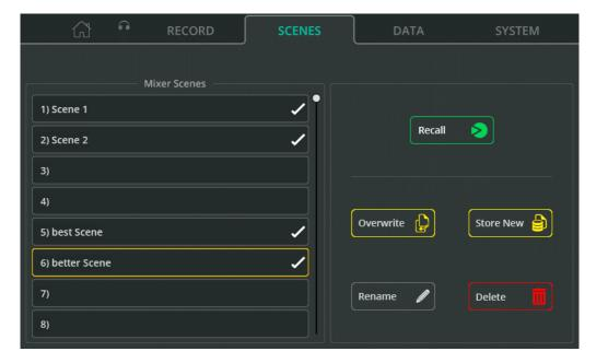
Scenes are used to store and recall the mix state of the CQ including all processing and send levels. 100 scene slots are available.
