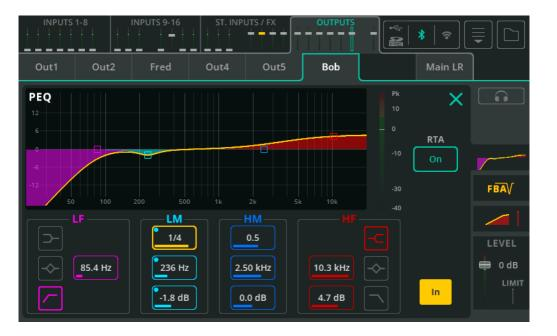
The 4-band Parametric Equaliser enables adjustments to the tone of the signal by cutting or boosting around different frequencies.
