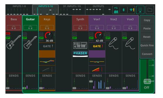
Any Quick Channel can be converted to a Complete Channel at any time without any change to the audio.
