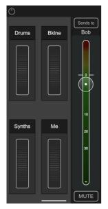
The main screen displays the overall output level on the right, with the ability to select the output being controlled above this, and a mute at the bottom.
