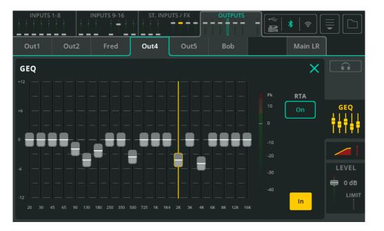
A GEQ is used to cut or boost specific frequencies in the signal.
