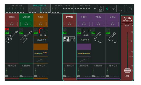
The bank view displays one of four banks at a time, each showing up to eight input, FX or output channels. Switch between banks using the tabs with mini faders and meters at the top (when using a CQ-12T or CQ-18T touchscreen) or bottom left (when using the CQ-MixPad app).
