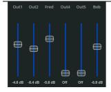
**13.** Adjust send levels to Main LR, other FX Units and Outputs 1-6 as required, so the FX is heard only where it should be.
