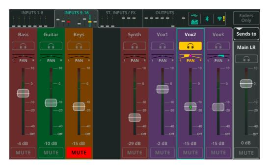
The Fader screen displays up to eight channels at a time. Use the mini fader tabs at the top (touchscreen) or bottom left (CQ-MixPad) to switch between the 4 banks of channels. Use the **Faders Only** button at the top right to either show channel Listen, Pan and Mute controls, or longer faders with no controls.
