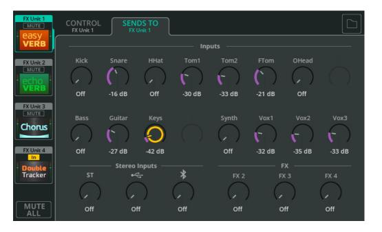
When FX units are in Shared mode, use the **SENDS TO** tab to view and adjust channel send levels to the selected FX unit.
