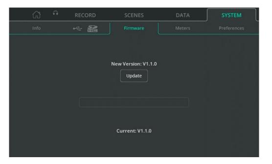
Shows the firmware currently installed on the unit at the bottom of the screen along with the firmware found on a connected USB drive at the top.
