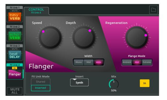
A Flanger folds the signal back on itself and uses a very fast modulated delay to create a shifting metallic effect.
