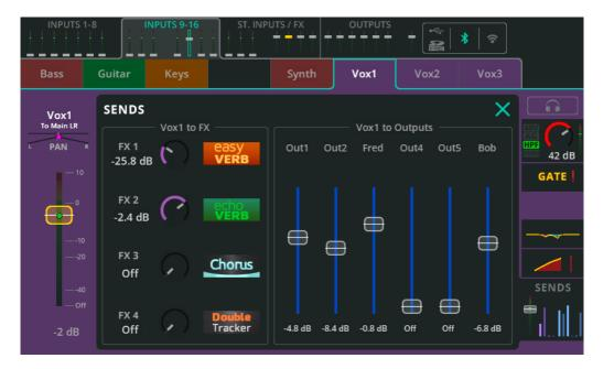
The SENDS section shows all send levels from an input or FX channel to all possible destinations.
