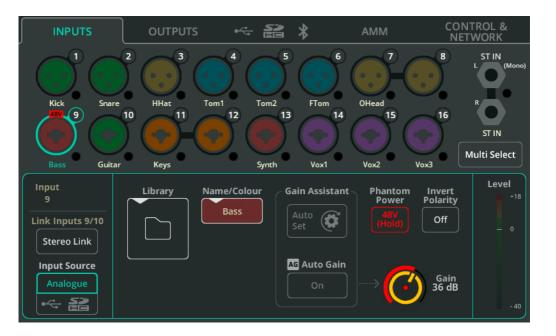
Input sockets are shown at the top of the screen, matching the hardware layout. Each includes a Chromatic Meter to show input signal.
