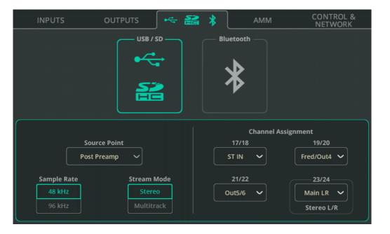
**Source Point** – Choose whether the signal being sent to USB/SD from input channels includes no input channel processing, some processing, or all processing.
