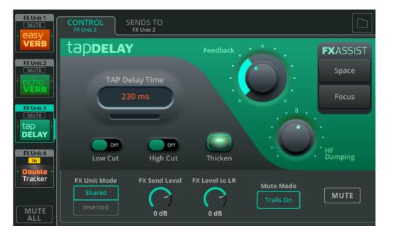
Tap Delay is a single delay which allows the speed of the repeats can be set using taps on screen or using a Soft Key.
