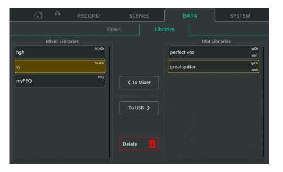
The CQ can have up to 128 User libraries stored at any time. These are included when storing or recalling an entire Show, but can also be stored or recalled individually using a USB drive.
