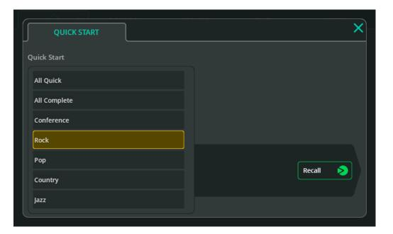
The Quick Start button (in the first **HOME** screen tab) opens a list of factory templates for use as the starting point for some typical mixer applications.
