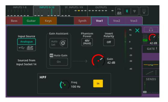
**Input Source** – Select Analogue to source the channel from the analogue sockets or select USB/SD to source from USB drive and SD card.
