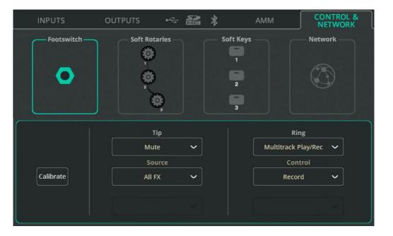
A single footswitch using a TS (Tip, Sleeve) connection or a dual footswitch using a TRS (Tip, Ring, Sleeve) connection can be used with CQ.
