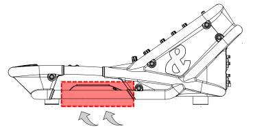
Leave adequate space for ventilation (~) at the sides of the mixer in the area indicated.
