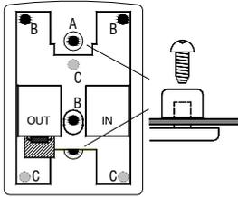
To change them, first remove the three screws (B) and unplug the top PCB. Remove the three screws (C) and lift the lower PCB away. Rotate the switch caps into the required position. Reassemble the module taking care to correctly align the inter-PCB connector.
