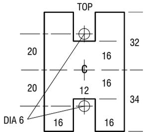
The assembled module fits into an 'H' shaped cutout in the centre of the mounting plate. The module is held using the two screws with plastic clamps provided (A). Unscrew these from the module first. Dimensions are in millimetres below.
