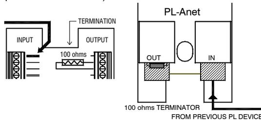
**Connection to the iDR** The PL-Anet network plugs into the iDR unit using an RJ45 connector. This is wired to the 568B scheme. The PL-Anet port provides the RS485 serial communication and +20V DC power to the chain of PL modules. The device addresses are automatically allocated per type in the order they appear in the PL-Anet chain.
