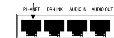
**PL-Anet** is the proprietary Allen & Heath system for daisy chaining remote controllers. It is an RS485 serial connection that uses CAT5 STP cable to communicate between devices over long distances. PL-Anet only works with Allen & Heath **PL** devices. The connection includes +20V DC to power the connected devices. The **iDR-8** port is shown here.
