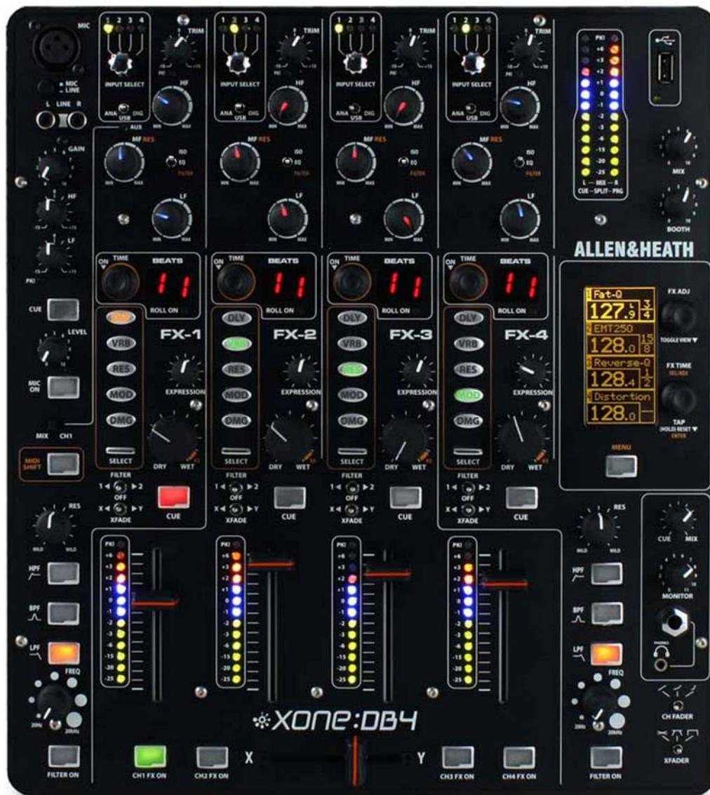
**MIDI CONTROL:** All controls (except Mic and Phones level) send MIDI data and the mixer can double up as a MIDI controller via the MIDI shift button, allowing the Loop and FX selection controls to send MIDI data without changing the mixer settings.
