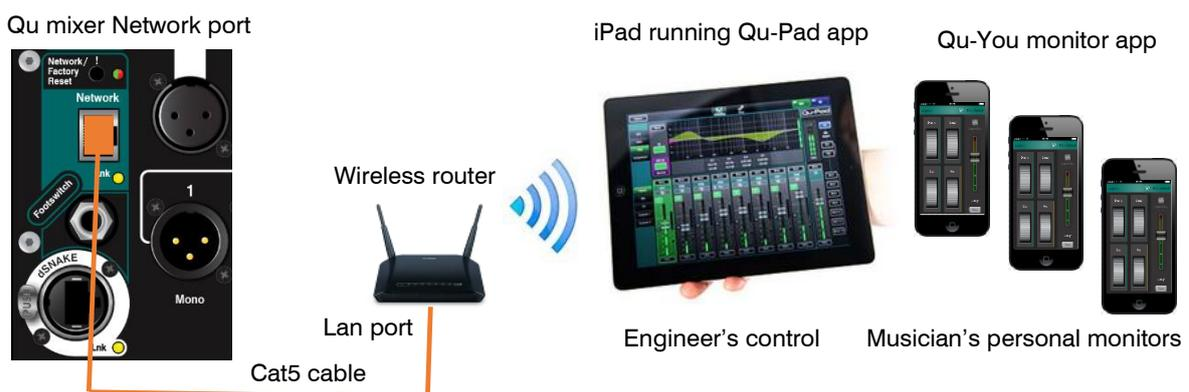
**Wireless router setup** – Connect the router to a PC or Mac using a Cat5 cable. Follow the instructions provided by the router manufacturer to access its setup menus. Once set up, disconnect the router from the computer and then plug it into the Qu mixer Network port using a Cat5 cable.
