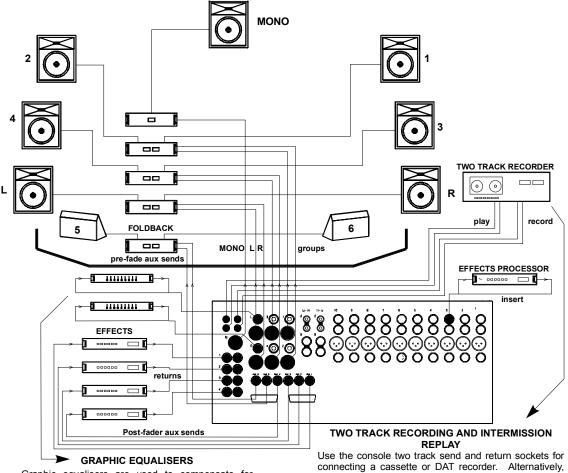
Graphic equalisers are used to compensate for adverse room acoustics. These devices help reduce acoustic feedback and enhance the clarity of the sound.
