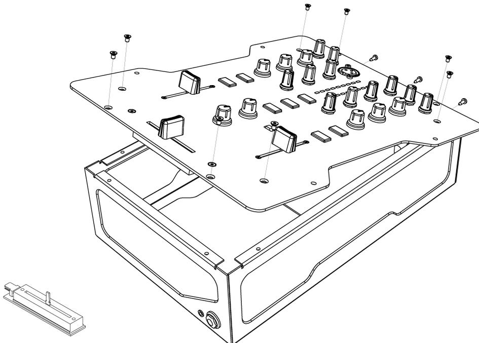
Whilst holding the cross fader, using the T8 torx driver, remove the 2 screws either side of the crossfader unit from the front panel.
