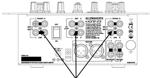
REMOVE THE T10 SCREWS ARROWED
